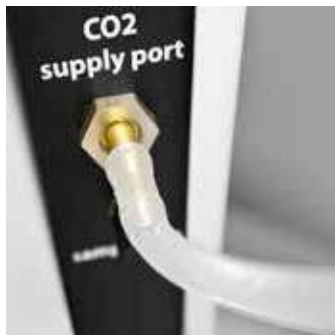
Simple CO 2 tank connection
